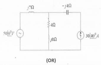
**Q10** By Using Thevenin's theorem, find the current through the  $4\Omega$  resistor?
