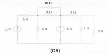
**2.** Find the value of current for the network shown in the figure by using Star- delta / delta- star transformation?
